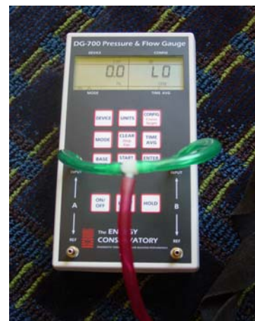
Figure 1161-1: Manometer set-up for exhaust fan flow hood
