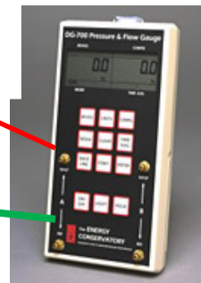
Figure 31211-1 Manometer set-up for WCD test
