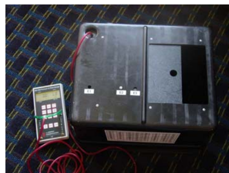
Figure 1161-2: Manometer and exhaust fan flow hood – flow hood is set to the E2 opening
