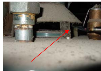
Figure 3122-1: Appliance passes spillage test
