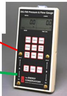
Figure 31211-1 Manometer set-up for WCD test
