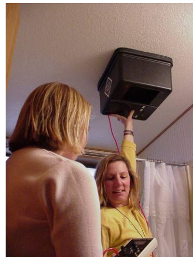
Figure 116-1: Exhaust fan flow meter being used to measure bathroom exhaust fan flow
