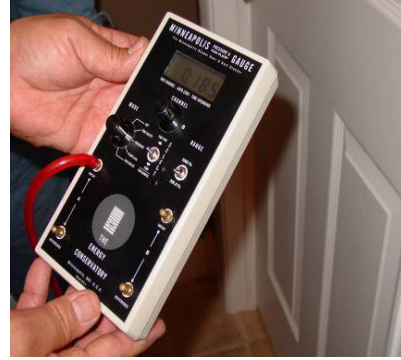
Figure 1152-1: Duct induced room pressure is 18.5 Pa!
