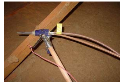
Figure 2122-12: 2-part spray foam gun secured to broom stick with string attached to handle
