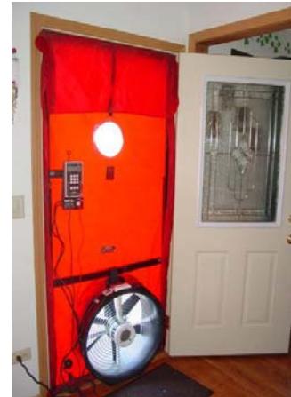
Figure 1112-1: Blower door set-up
