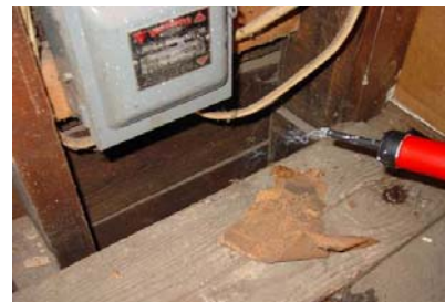
Figure 2121-1: Smoke being drawn down an open study cavity indicating leakage to the inside
