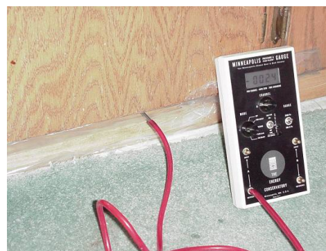
Figure 1141-1: Toe-kick sealed with duct mask tape; pressure pan reading of 24 Pa!
