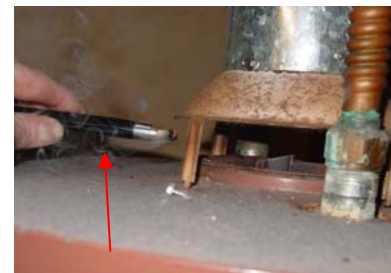
Figure 3122-2: Appliance fails spillage test
