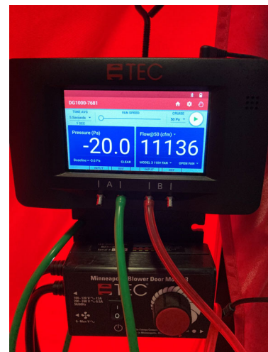
Figure 11121-1: CFM50 is displayed when 50Pa cannot be achieved in a home
