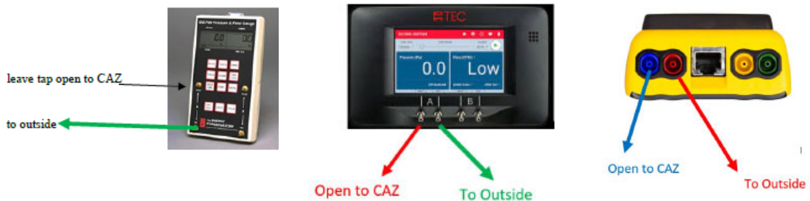
Figure 31211-1 DG700, DG1000 & DM32 manometers set-up for WCD test. Note that hose to CAZ not necessary if readings are being taken in the CAZ
