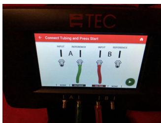
Figure 1112-2: Hose connections for the DG1000, DG700 and DM32 manometers
